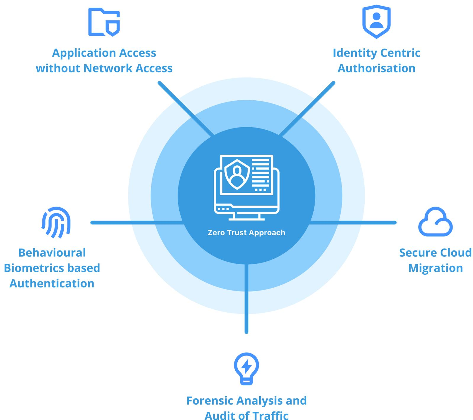
The traditional security model uses network perimeters which divide users and devices into 2 groups: those on the 'inside', deemed to be 'trusted', and gaining unrestricted access to resources within the network, and those on the 'outside' which are untrusted. This system of assigning excessive trust by default, as an entitlement, has an inherent problem. Once the network perimeter is breached, attackers can move laterally through the network, accessing and exploiting all critical resources.
